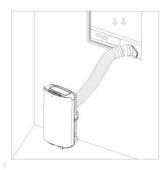
Keep the hose as straight as possible, avoid dips where the moisture from the exhaust air can condense and fill the tube with water. Do not allow the hose to be crushed.
