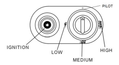
1) Push and hold the control knob down at the pilot position for 10 seconds. Whilst still holding the control knob down, press the ignition button several times until a pilot flame appears along with the centre ceramic plate being lit.
