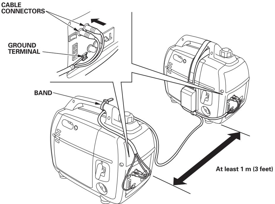
3. Connect the ground terminal of one generator to the ground.
