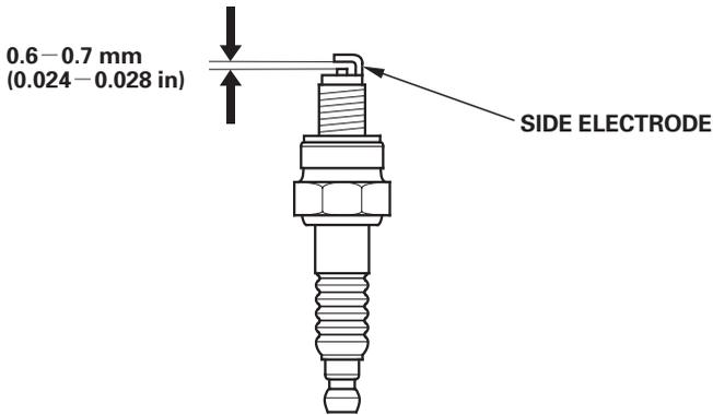
7. Install the spark plug carefully, by hand, to avoid cross-threading.
